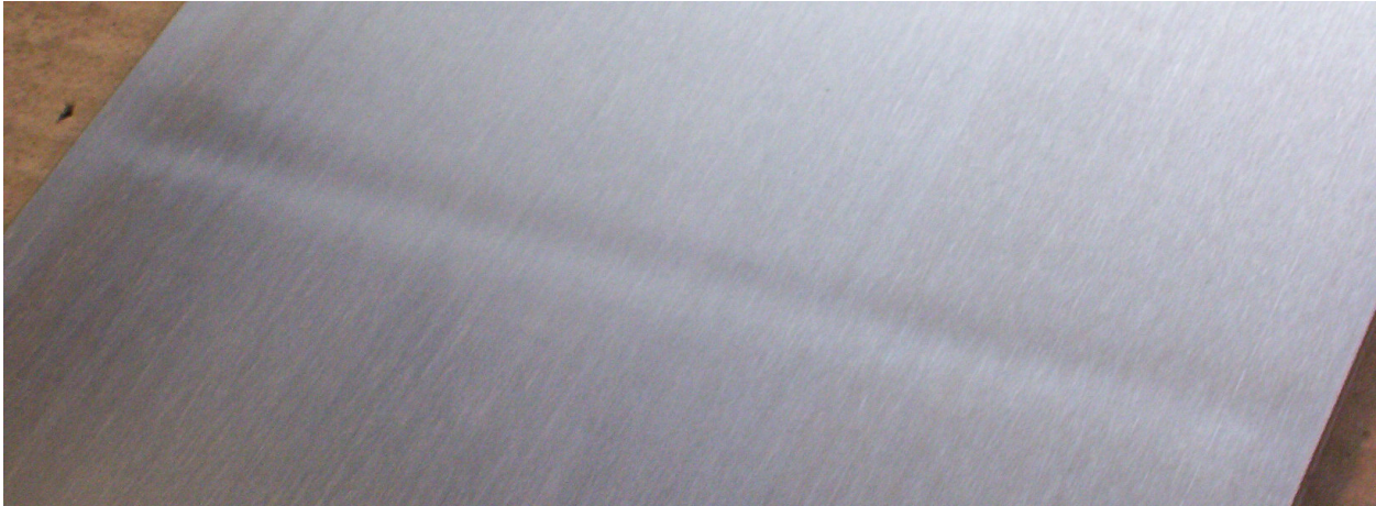
Fig. 1 - Sanding mark on polished stainless steel.
